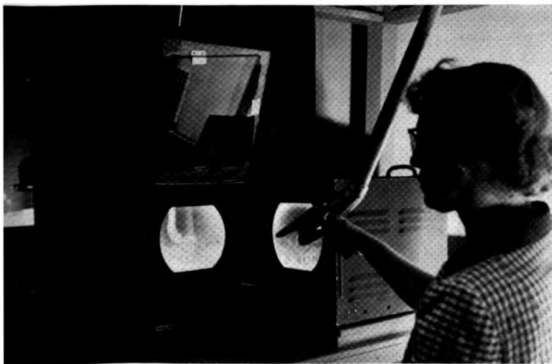
Credit: University News Service Manipulators are used for handling radioactive substances at a safe distance. The operator is viewing her work by 3-D television; there are no mechanical links, just a single coaxial cable, between the operator and the operation.
