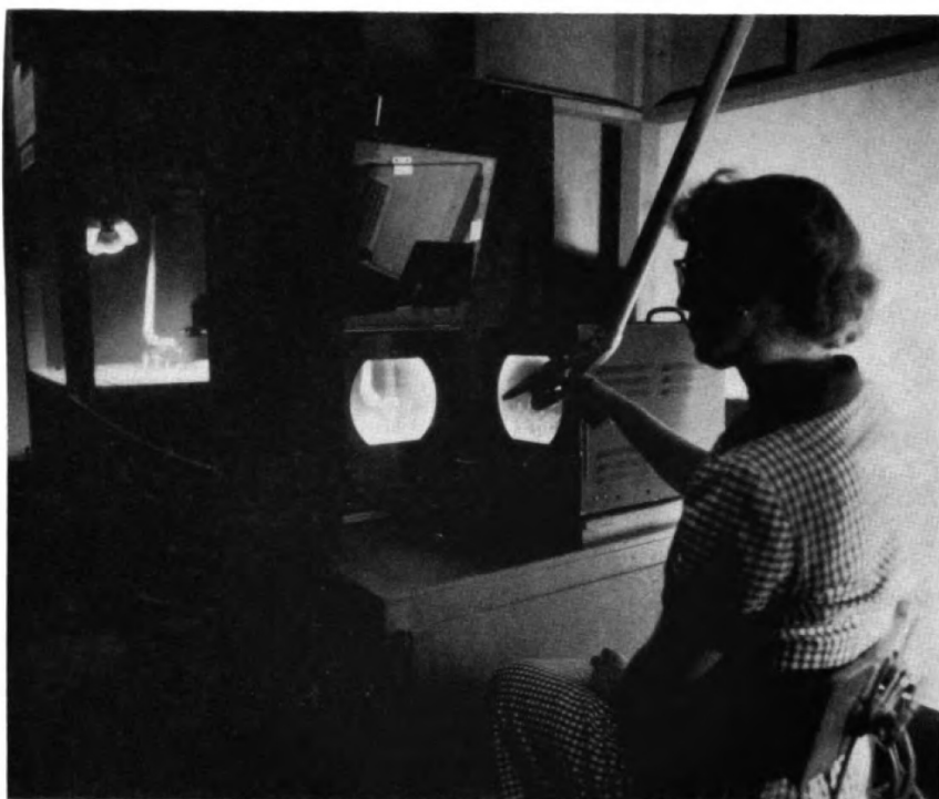
Demonstrating the agility that can be achieved in using mechanical hands, this worker at the Phoenix Project watches her actions on the television screen.
