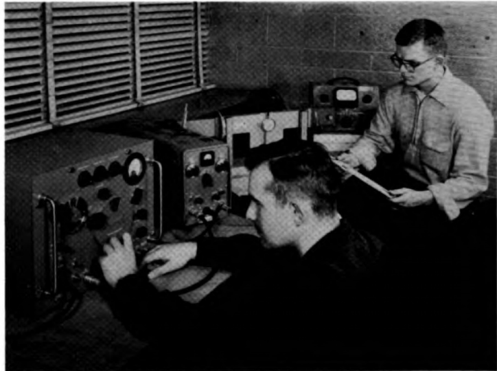
Measurement of the power Output and gain of a Wideband Traveling Wave Amplifier.
