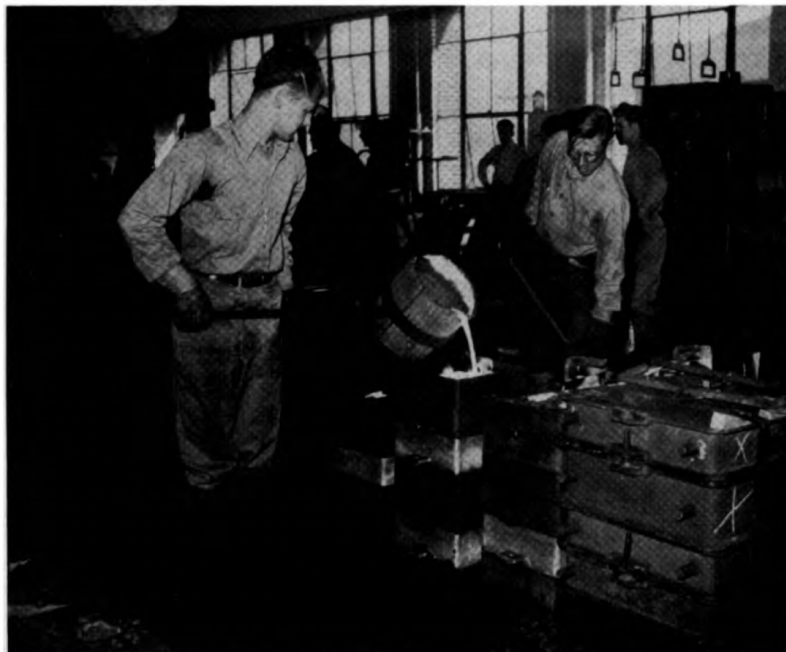
Metallurgical engineering students have a well-equipped metals laboratory and foundry. Students are shown pouring an experimental mixture of alloy steel into a casting mould.
