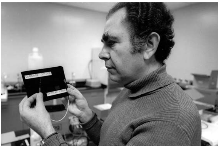
Jerome S. Schultz with his invention of a glucose sensor optode. The sensor chemistry is encapsulated in a single dialysis fiber sensor chamber placed at the end of a single optical fiber (left hand). The magnitude of fluorescence produced in the sensor chamber is directly related to the glucose concentration in the fluid in which the probe is placed, and is measured by a photometer attached to the other end of the optical fiber (right hand).
