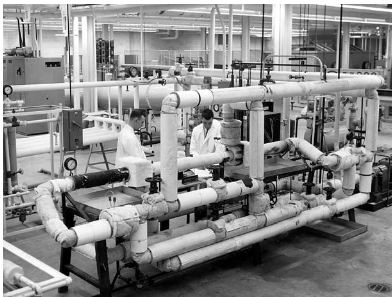
John G. Lavin and Dale E. Briggs, measuring heat-transfer rates and bond resistances of finned tubes at high temperatures.
