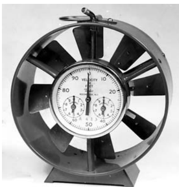
Anemometer used in finned-tube wind-tunnel tests, 1955.
