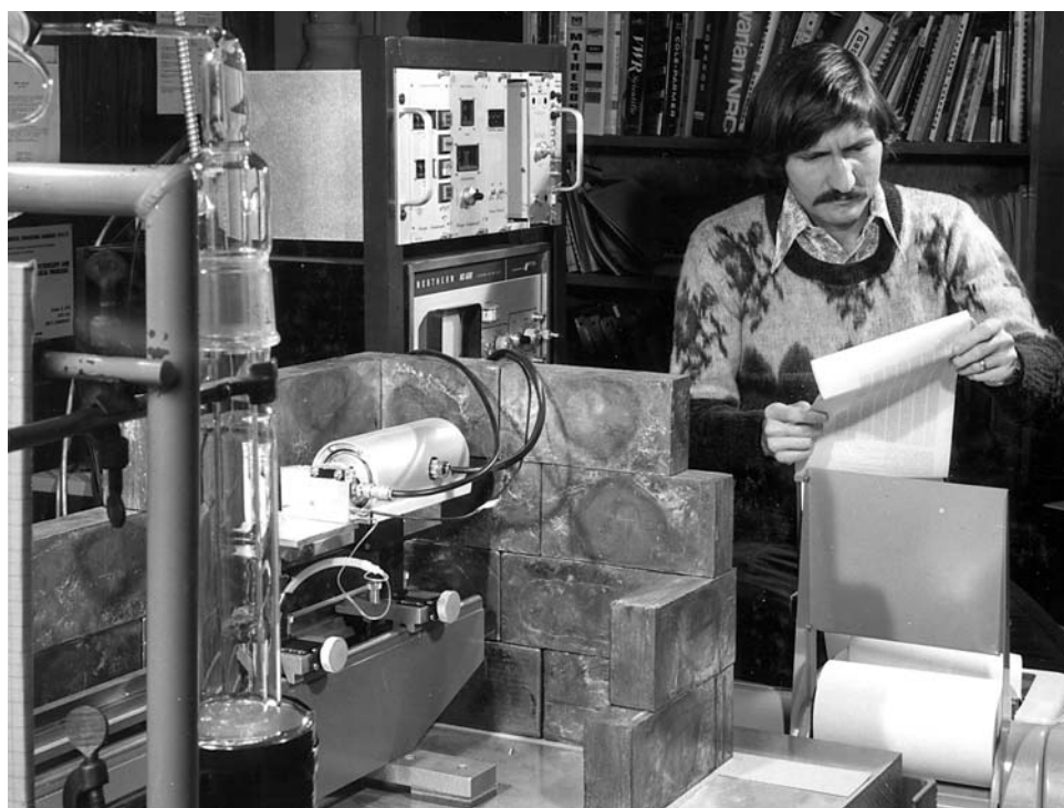
James G. Goodwin (Ph.D. 1976), involved in his research into the decarburization of Fe thin films by hydrogen, working with Prof. Parravano. The equipment used a Mössbauer spectrometer to detect conversion electrons. Using this detection system, the nature of the carbides present and their amounts could be determined as a function of time and temperature.
