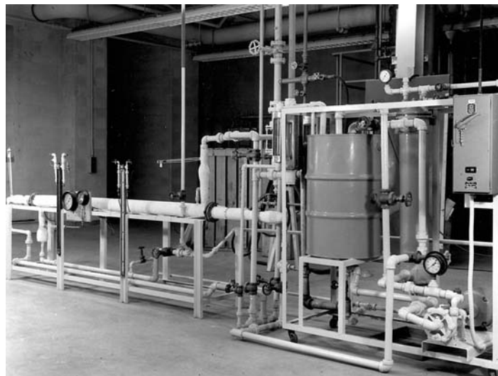
Concentric-pipe heat exchanger is a 9-ft test length fabricated from 2-in. pipe, used for studying heat transfer and pressure drop characteristics of the inside of tubes with internal extended surfaces or turbulators.
