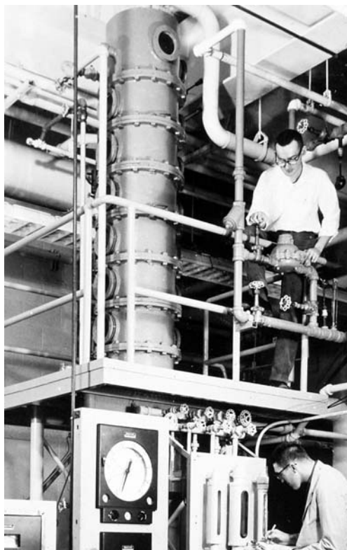
The 18-inch ethanol/water distillation column, which was one of the experiments in the ChE 460 laboratory on the first floor of the G.G. Brown Building. Doctoral student Robert Norman is on the upper level.
