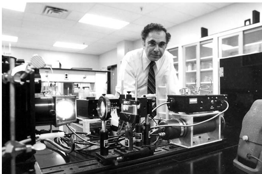
Jerome S. Schultz with his light-scattering instrumentation that was used to determine the effects of shear on the kinetics of fibrin aggregation. This was one aspect of his NIH-supported project to develop a fundamental understanding of blood coagulation in devices such as artificial kidneys and heart-assist pumps.
