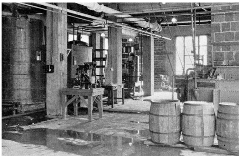
A detail of the second floor general laboratory showing the crystallizer on the right with a little centrifuge to the left. In the left-hand corner are tanks, and in the rear a water-softening unit of the zeolite type.
